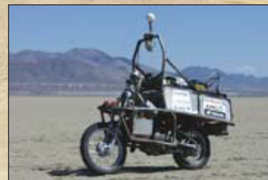
GHOSTRIDER ran unassisted for 20 miles at a time in desert testing.
